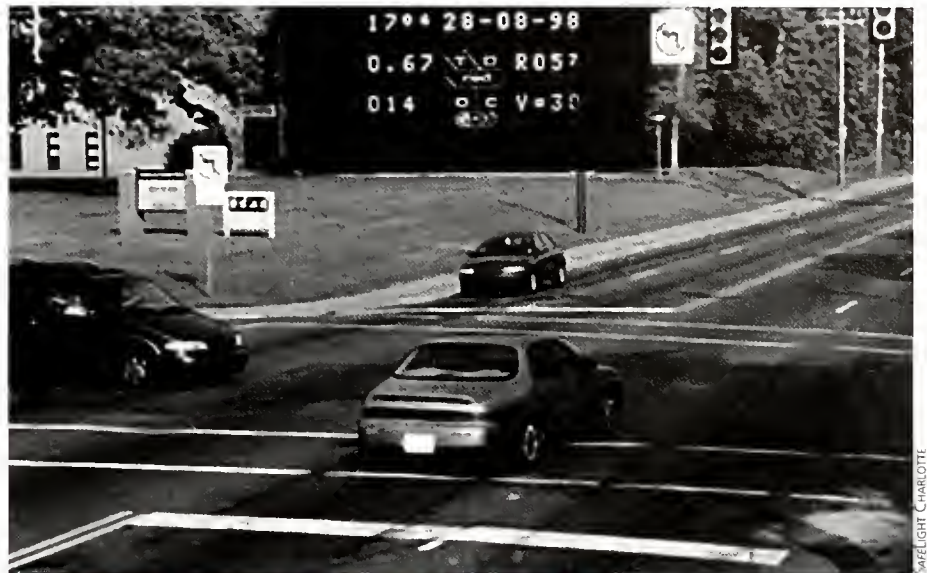
The automated camera takes two photos of the vehicle and the light, one before the vehicle enters the intersection, and one after. Above, the second photo, with relevant data superimposed: "17 04" is the time of the violation; "28-08-98," the date it occurred; "0.67," the elapsed time between the two photos; "R 0 57," the total elapsed time of the red phase at the time of the second photo (here, 5.7 seconds); "014," the violation number on the camera film; and "V = 30," the vehicle speed.
