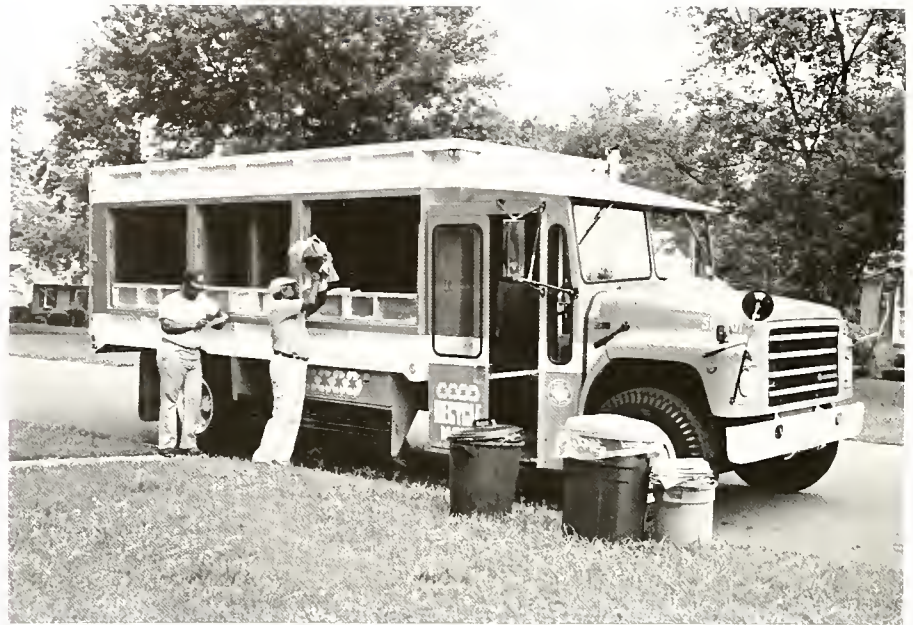
Recyclable materials are collected in trucks having storage compartments for three different materials.
