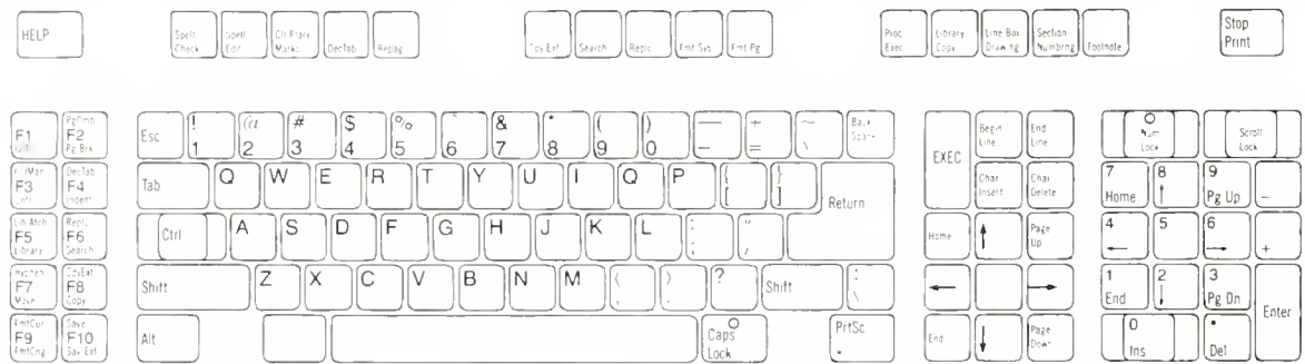
A. Specialized Word Processing Keyboard. Has labeled function keys, additional labeled command key, separate cursor movement keys, larger shift, and return keys.
