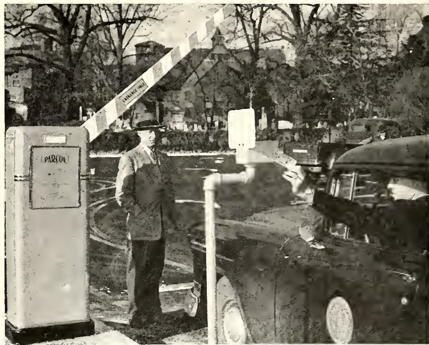
Monthly parking lot with electronically controlled entrance and exit gates.
