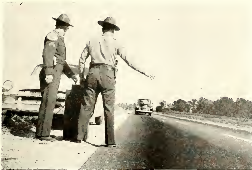
These patrolmen have clocked a speeding car on the speed watch, and are flagging him to a stop. The speed clock device shown between the patrolmen registered the speed of the motorist as he passed over the two speed watch tubes laid across the road a few hundred yards from the officers.
