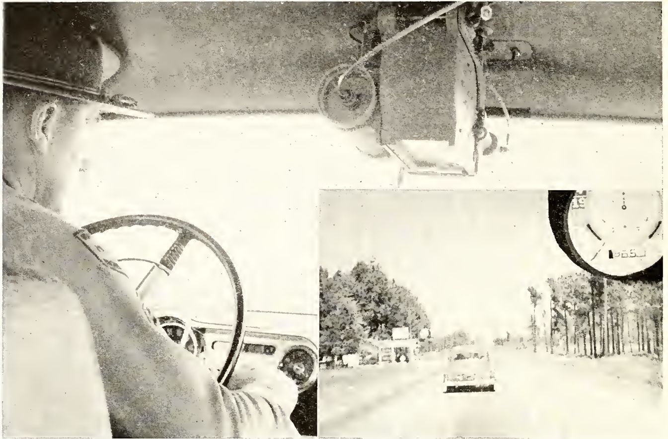
The patrolman shown above is using one of the Patrol's camera-equipped cars to photograph and clock the speed of the car ahead of him. The camera appears at top center of the large picture, lens against windshield. The inset picture was made by the camera, and provides photographic evidence that the car ahead was traveling at 70 miles per hour.
